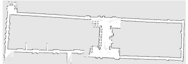
Fig. 3. A map obtained by integrating scans from a LRF. Picture courtesy of Univ. of Freiburg, Germany
