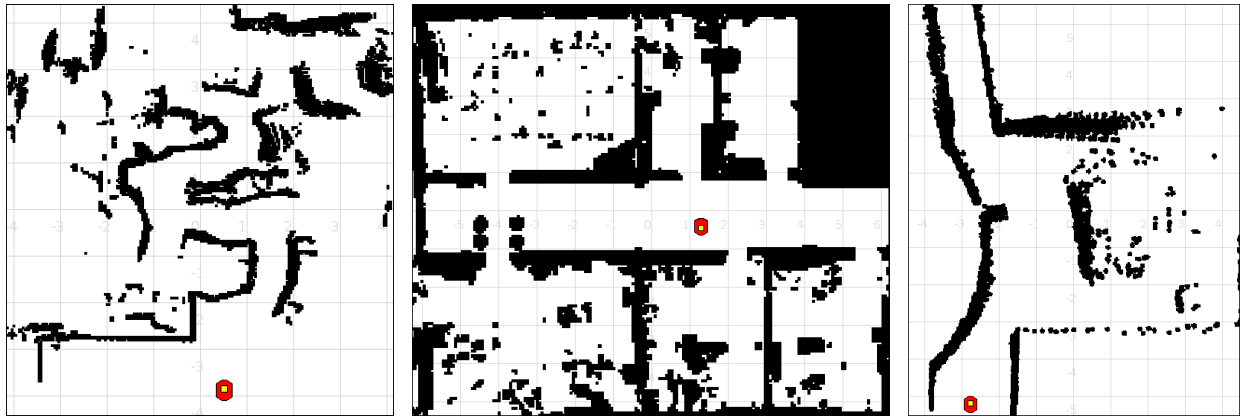
Fig. 1. Three maps taken from the benchmark database, showing also the robot starting pose
