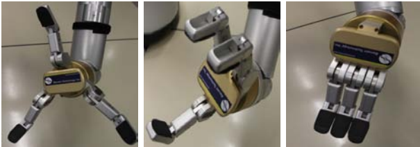
Fig. 1. Different grasp configurations can be combined with different grasping point selection methods.
