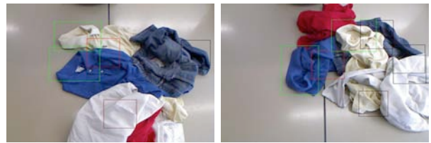
Fig. 4. Perception: a polo collar detector is used to find this distinctive part in the image. Grasping at this known part speeds up the task of leaving the cloth in a known configuration as specialized actions can be triggered.
